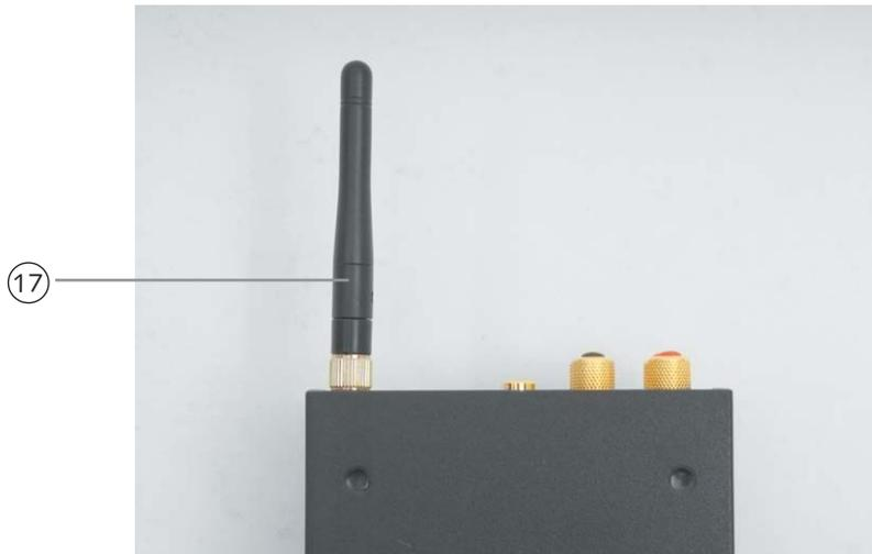
**ATTENTION:** Never operate your CD 3500 wireless and transceiver without the antenna screwed on as this may damage or even destroy the transmitter and receiver modules.
